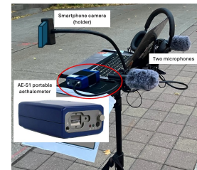
Fig. 3: Instrument deployed for user study, using a microaethalometer as ground truth
